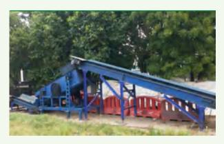
Vibro-Feeder used at the Material Recovery Facility at Jhajjar Power Station.
